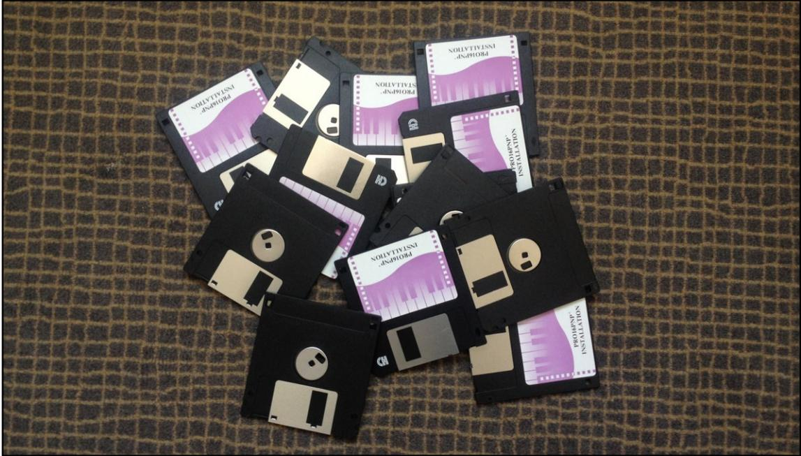
A **floppy disk**, or **diskette**, is a [disk storage](#) medium composed of a disk of thin and flexible [magnetic storage](#) medium, sealed in a rectangular plastic carrier lined with fabric that removes dust particles. Floppy disks are read and written by a **floppy disk drive** (FDD).
