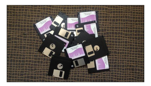
A **floppy disk**, or **diskette**, is a <u>disk storage</u> medium composed of a disk of thin and flexible <u>magnetic storage</u> medium, sealed in a rectangular plastic carrier lined with fabric that removes dust particles. Floppy disks are read and written by a **floppy disk drive** (FDD).
